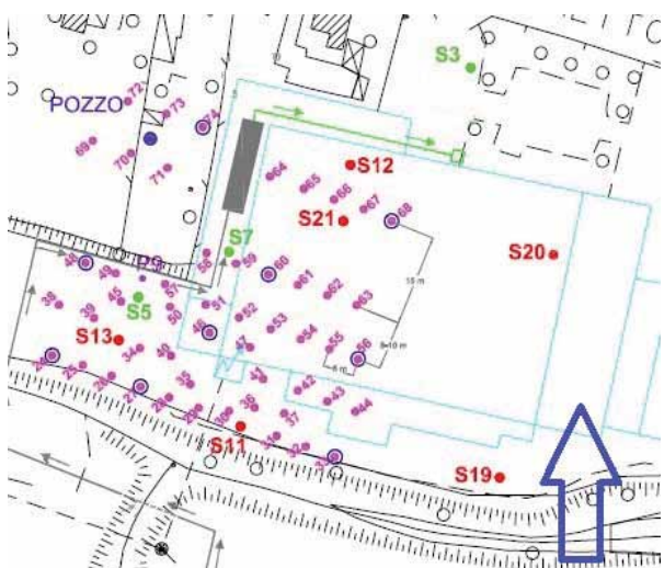
Fig. 5 - Grid of the injection points (in lilac) and monitoring points (in red, blue and green); the blue arrow represents the medium groundwater flow direction.
