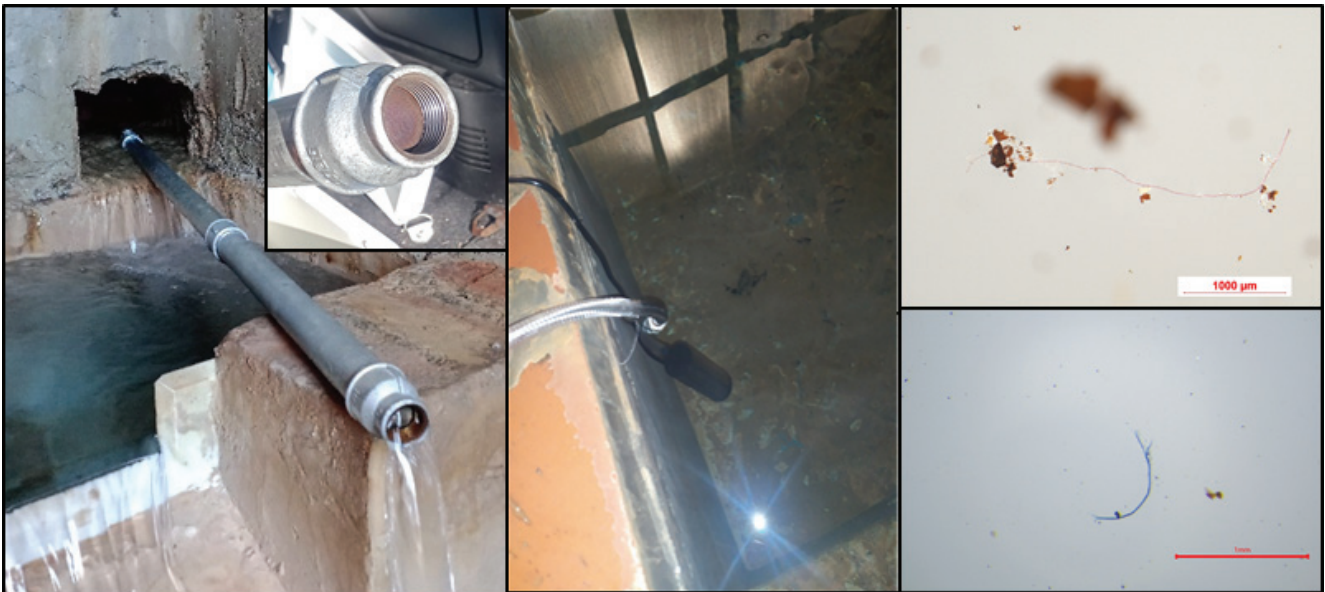
Fig. 4 - Typical source sampling with a metal branch tube and a 0.3 mm metal filter. Microplastics observed on the sample under a microscope.
