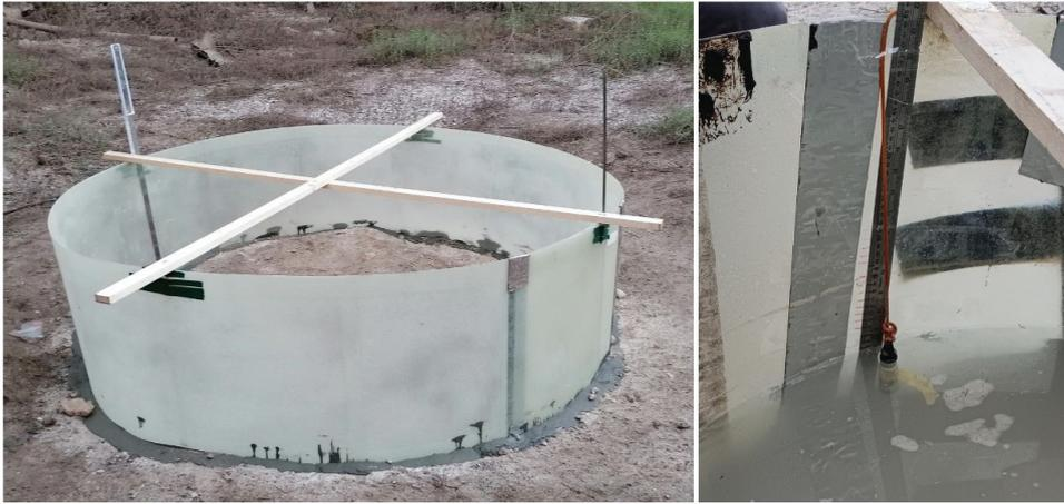
Fig. 4 - Infiltration ring installed directly on the outcropped rock at the bottom of the infiltration trench (left); CTD-Diver probe to measure the water level decrease in the ring during the infiltration test (right).
