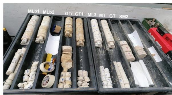
Fig. 3 - Rock blocks belonging to the Upper Coralline Limestone formation coming from three different areas (Ghajn Tuffieha, Mellieha and San Martin) from which were extracted the samples tested in the laboratory.
