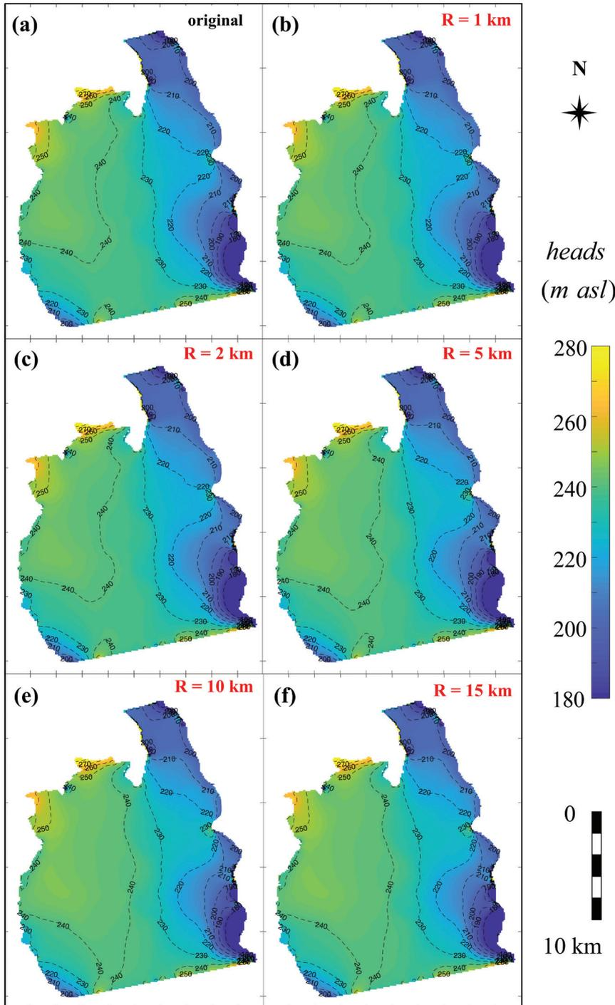
Fig. 6 - Piezometric levels for the domain of investigation simulated upon different conductivity fields.
