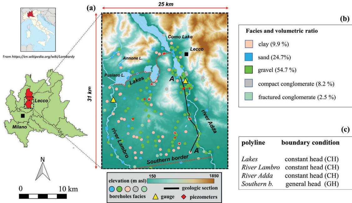
Fig. 1 - Sketch of the investigation domain and available data, (e.g. boreholes, piezometric head and geological section) (panel a). Geological facies volumetric ratios (b) and types of boundary conditions (c) are enclosed as well.
