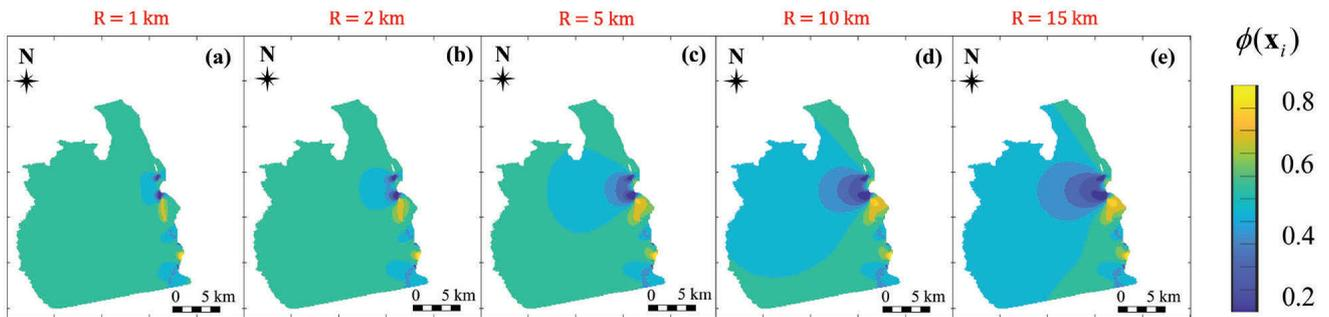
Fig. 4 - An example of porosity fields interpolated upon a simple kriging procedure for different correlation scales,  $R$ .
