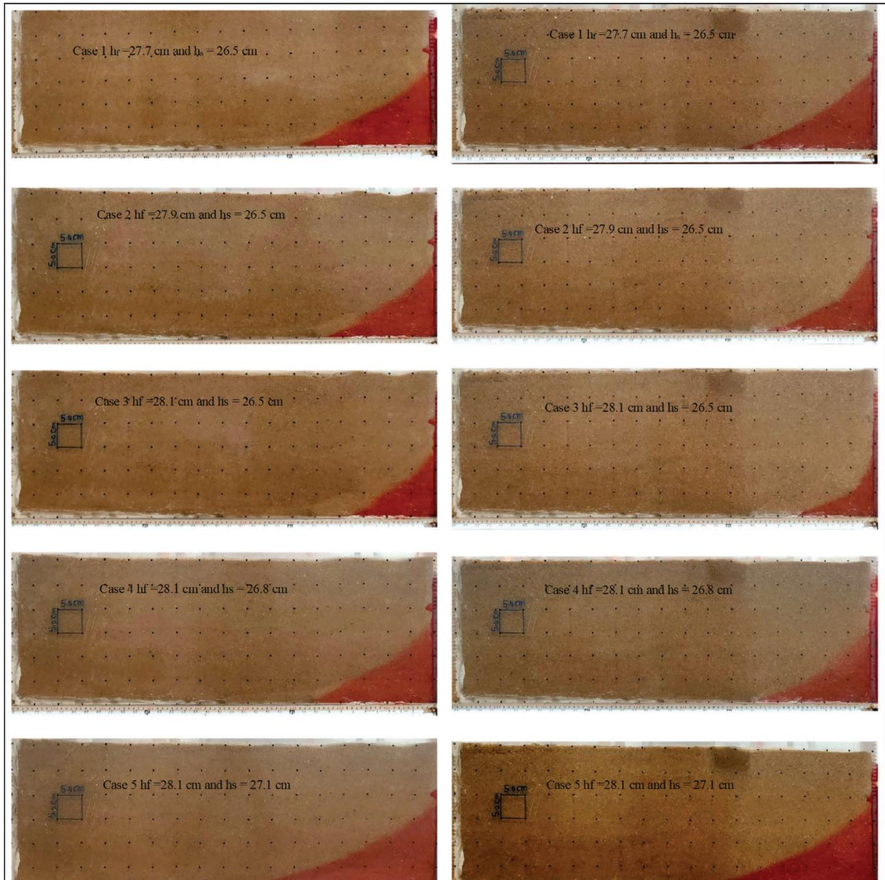
Fig. 5 - Experimental steady-state saltwater wedges for the low K (a) and the high K (b) aquifers.
