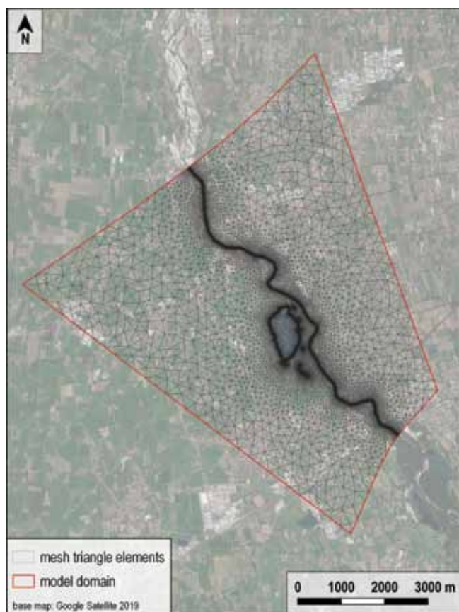
Fig. 5 - Finite element model mesh.
