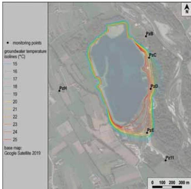
Fig. 8 - Hot water plume generated by the lake at peak temperature.
