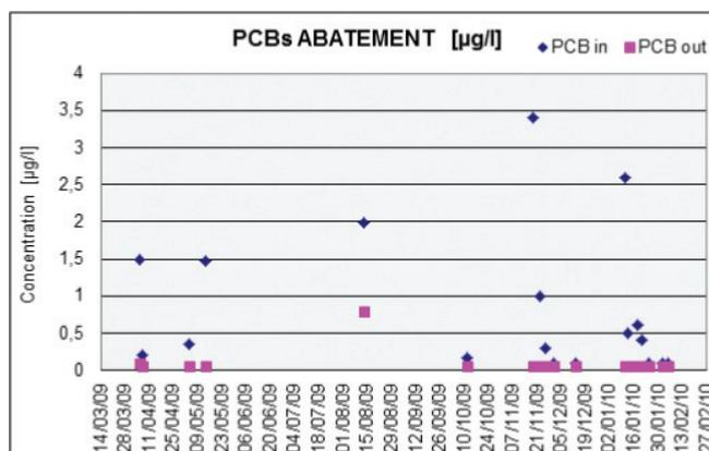
Fig. 9 - PCBs input-output system concentration monitoring.
