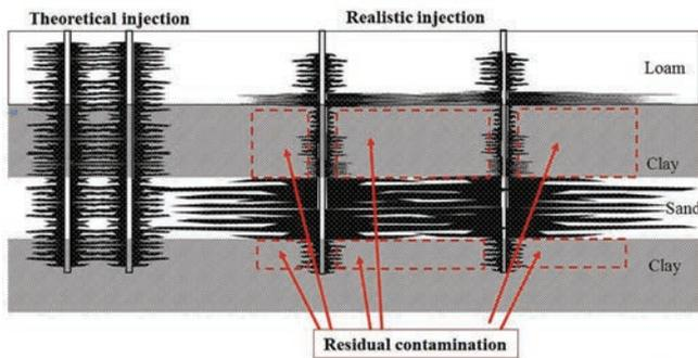
Fig. 4 - Differences between theoretical and actual injection radius due to soil heterogeneities. Different injection radii are actually obtained due to soil heterogeneities (the lower the permeability, the smaller the radius of influence), thus leading to incomplete remediation of target areas.
