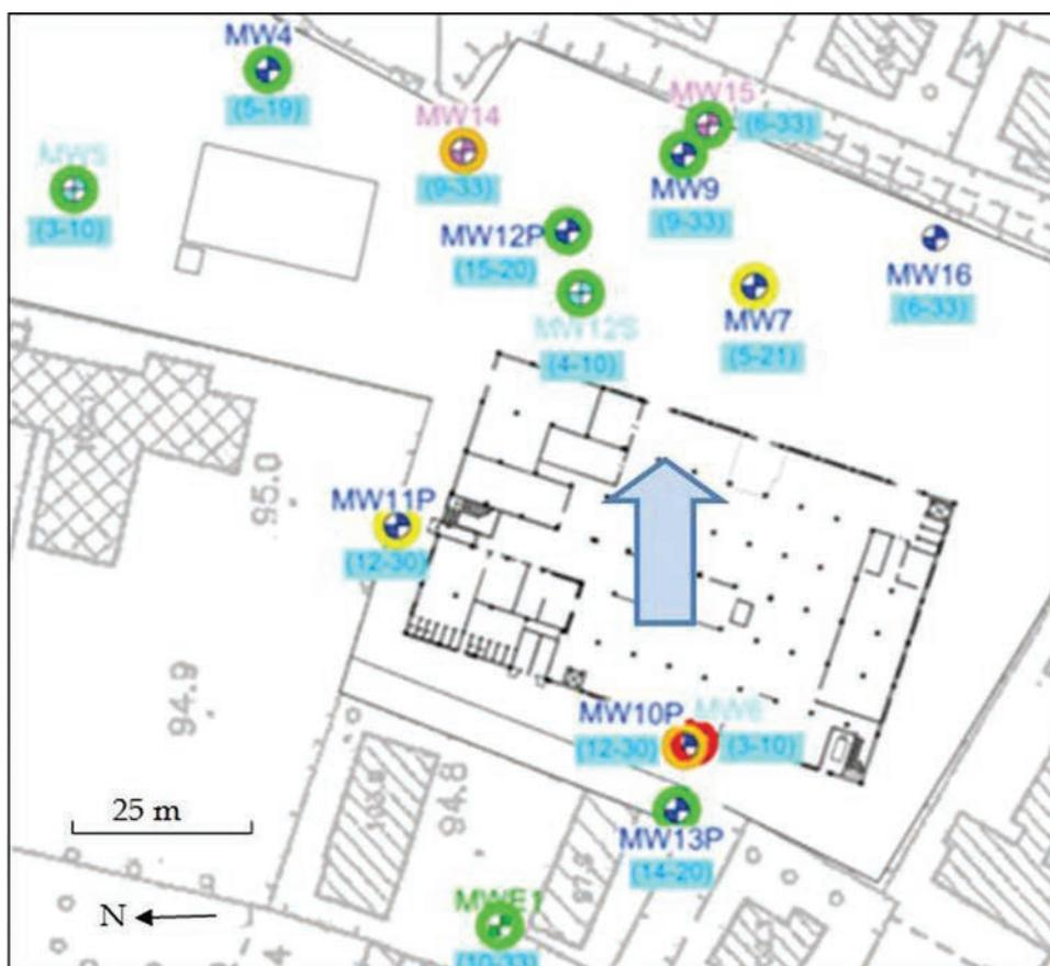
Fig. 8 - Site Groundwater Impacts. Monitoring wells (MW) names are shown (screened intervals in m bgl are reported in round brackets). Chlorinated impacts are shown in green (<10 µg/l), yellow (10-100 µg/l), orange (100-1000 µg/l), purple (1,000-10,000 µg/l) and red (> 10,000 µg/l) circles. Main groundwater flow is West-East. MW14 and MW15 are hydraulic barrier wells. The main production building is located just East of monitoring wells MW6 and MW10P.
