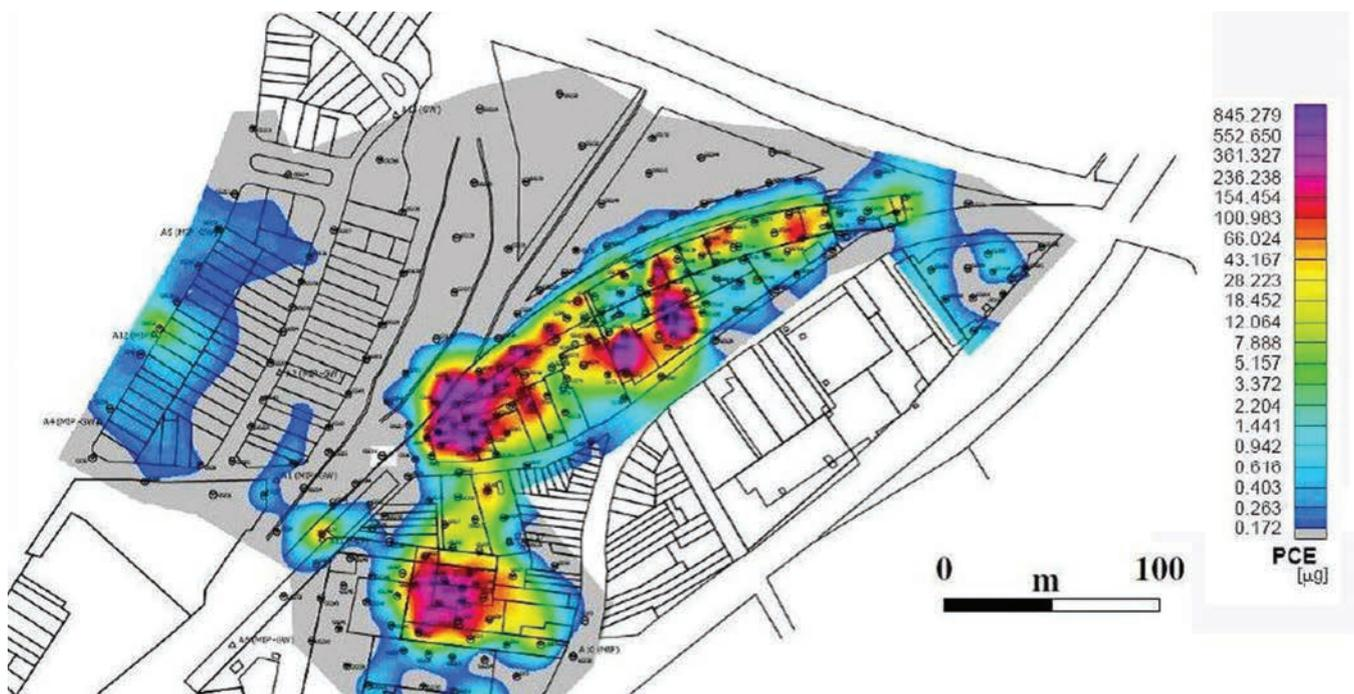
Fig. 6 - Passive soil gas samplers – Typical results of the investigation. The most impacted areas are shown in purple. Passive soil gas sampling data are reported in units of mass (as shown in the column on the right sector of figure), although concentration data can be in some cases calculated.
