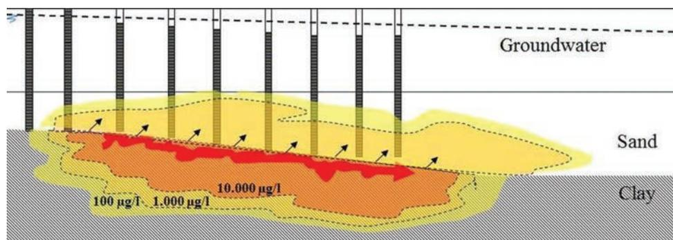
Fig. 3 - Rebound effect from low-permeability layers after remediation of high-permeability layers. If remediation activities are focused on high-permeability layers only, dissolution of residual contamination located in low-permeability layers may generate rebound effects.
