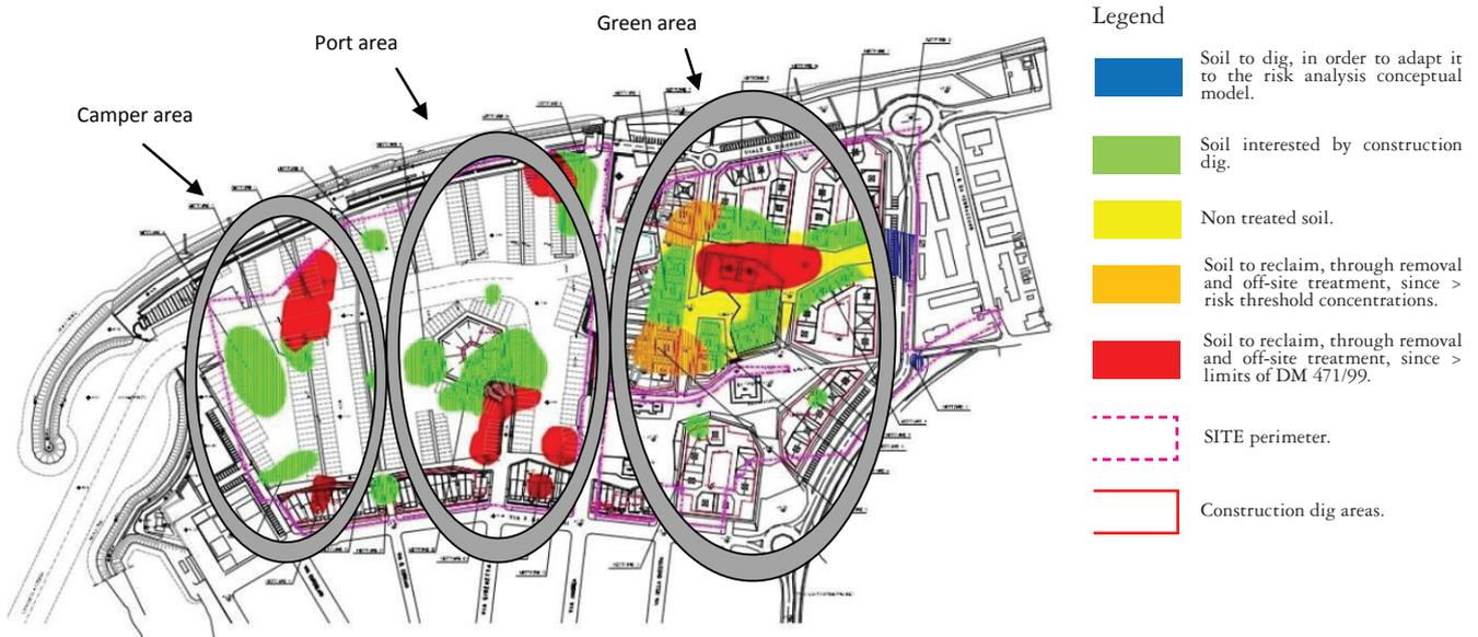
Fig. 1 - The area showing the sectors to remediate.
