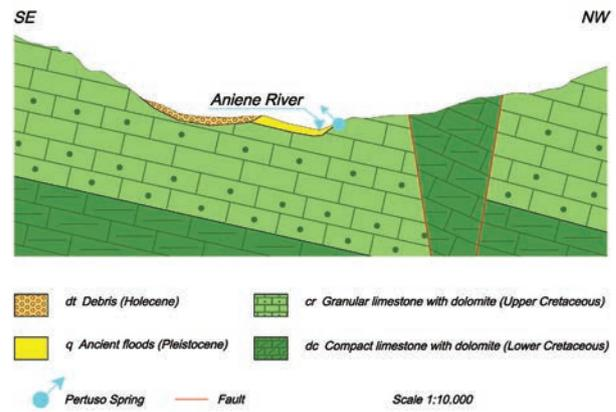
Fig. 2 - Geological cross section of the Pertuso spring.
