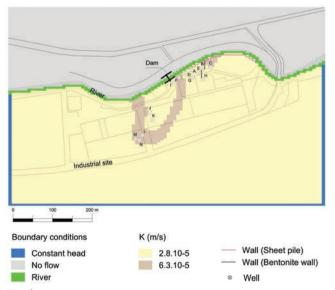
Fig. 4 - Model finite-difference grid, boundary conditions and bydraulic conductivity zones of Layer 1.
