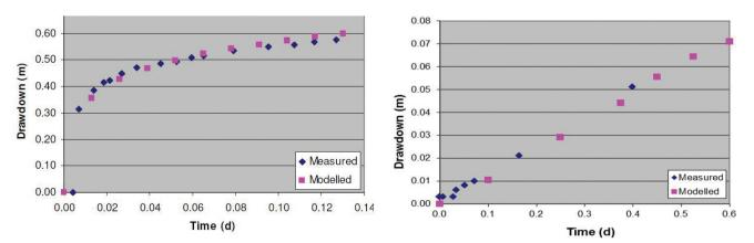
Fig. 7 - Model verification: simulation of well N pumping test.
