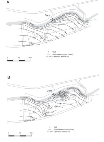
Fig. 6 - Modelled groundwater contours under static and abstraction conditions. Fig. 6 - Piezometrie simulate in condizioni statiche e dinamiche.
