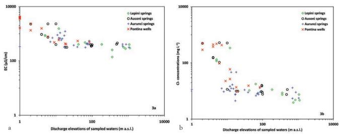
Fig. 3a, b - Levels of EC (a) and chloride (b) versus discharge elevations of sampled waters.
