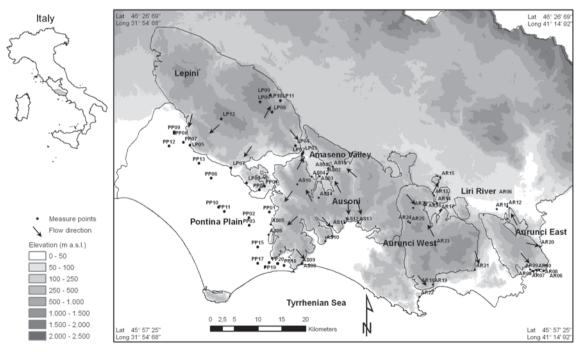
Fig. 1 -Site study area, location of springs and wells and the main directions of groundwater flow paths (LP: Lepini springs, AS: Ausoni springs. AR: Aurunci springs, PP: Pontina Plain).
